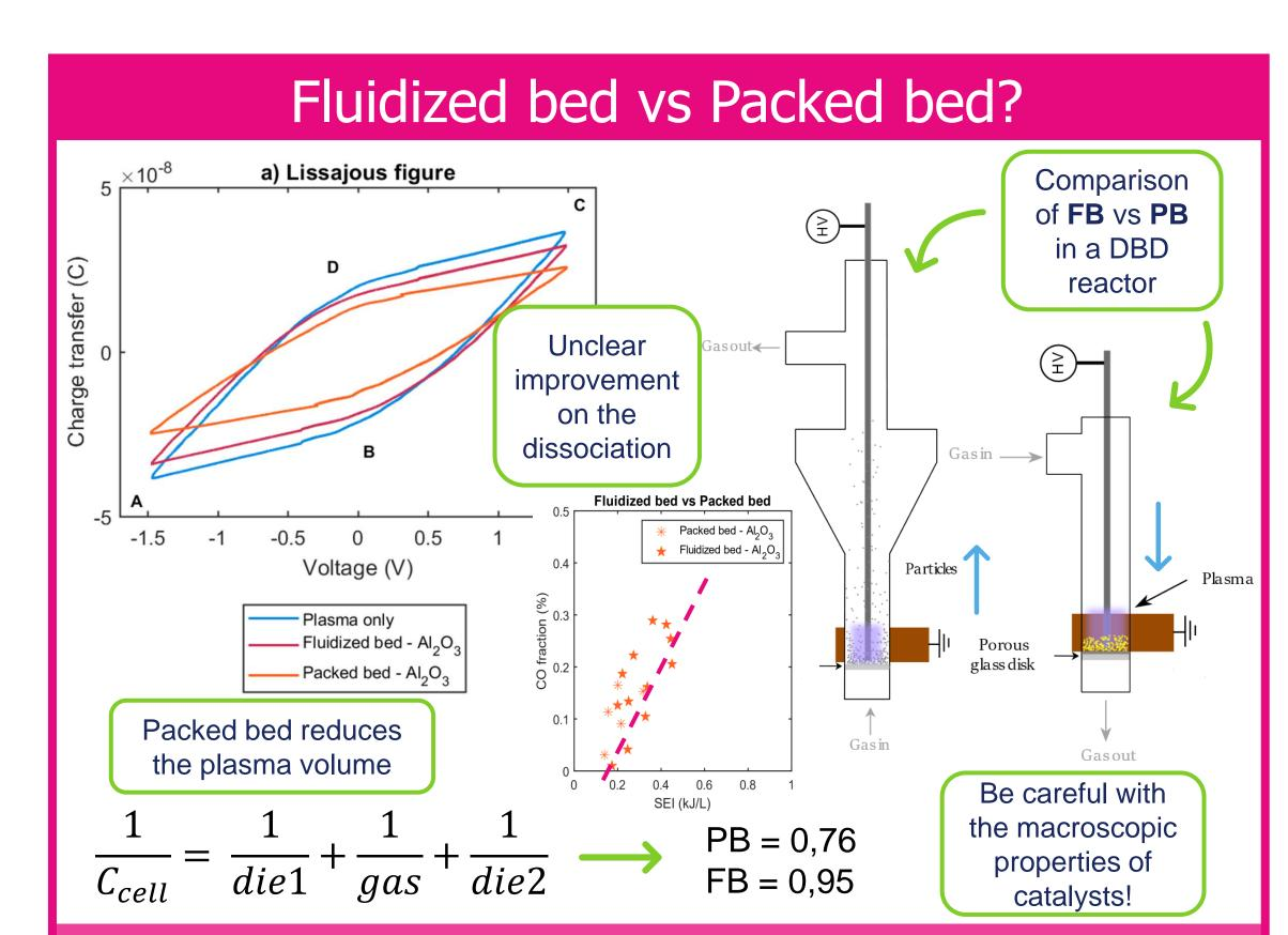
Movement of Al<sub>2</sub>O<sub>3</sub> particles affects less the ignition of filaments and therefore, the charge transfer
